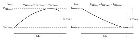
The temperature coefficient aV<sub>REF</sub> for the reference input voltage is equivalently given by the following expression.
