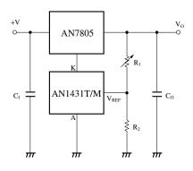
$$V_{\mathrm{O}} = V_{\mathrm{REF}} \left( 1 + \frac{R_{1}}{R_{2}} \right), \, V_{\mathrm{O(min)}} = V_{\mathrm{REF}} + 5V$$
