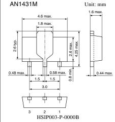
Note) The packages (SSIP003-P-0000 and HSIP003-P-0000B) of this product will be changed to lead-free type (SSIP003-P-0000S and HSIP003-P-0000Q). See the new package dimensions section later of this datasheet.
