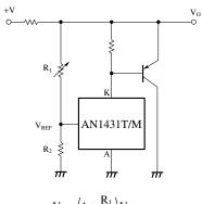
$$V_O = \left(1 + \frac{R_1}{R_2}\right) V_{REF}$$
