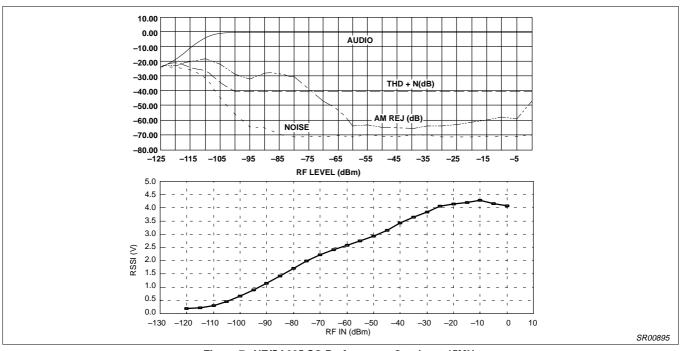
Figure 7. NE/SA605 SO Performance Graphs at 45MHz
