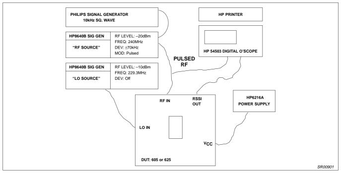
Figure 13. RSSI Speed Set-Up
