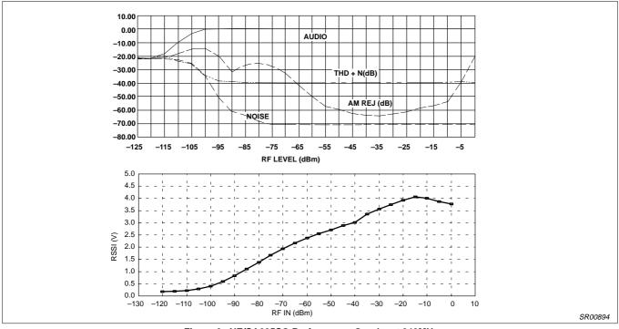
Figure 6. NE/SA605SO Performance Graphs at 240MHz
