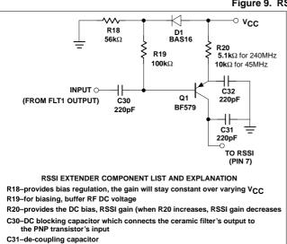
Figure 10. External RSSI Extender Circuit
