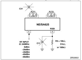
Figure 15. NE/SA625 RSSI Test Circuit Configuration
