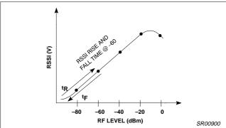
Figure 12. RSSI Cuve with Pulsed RF Levels
