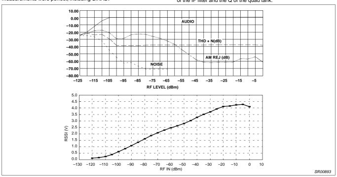
Figure 5. NE/SA625 SO Performance Graphs at 45MHz
