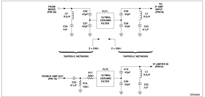
Figure 8. Matching Configuration for FLT1 and FLT2
