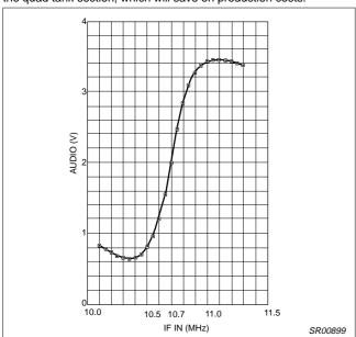
Figure 11. 10.7MHz Quad Tank S-Curve
