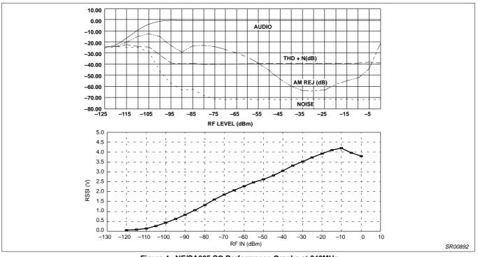
Figure 4. NE/SA625 SO Performance Graphs at 240MHz
