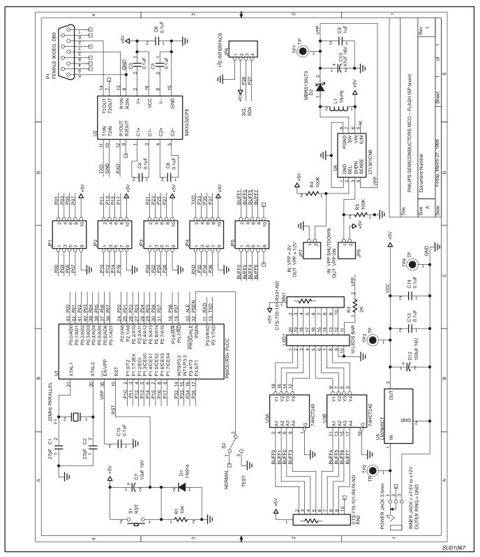
Figure 3. ISP Board Schematic Diagram
