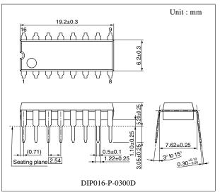
Note) The package of this product will be changed to lead-free type (DIP016-P-0300M). See the new package dimensions section later of this datasheet.
