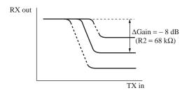
Figure 1. Variable width of attenuation
