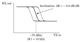
Figure 2. Operating point of attenuation
