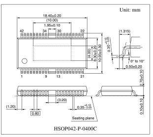
Note) The package of this product will be changed to lead-free type (HSOP042-P-0400G). See the new package dimensions section later of this datasheet.
