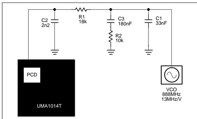
Figure 5. Loop Filter Circuit Diagram
