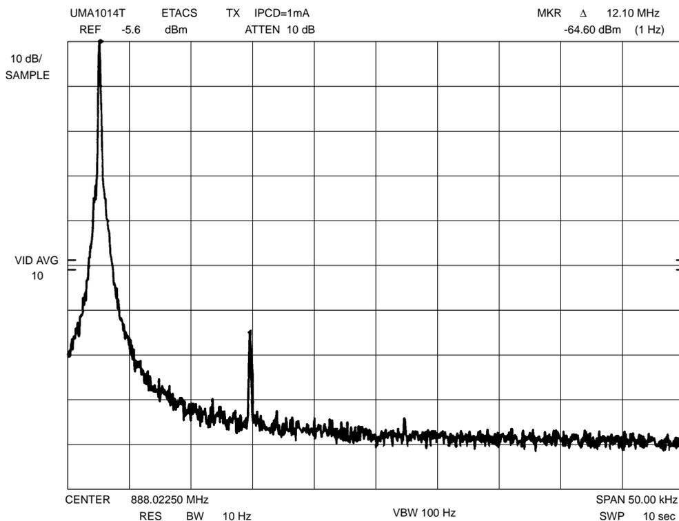
Figure 9. Typical Carrier Spectrum – 50kHz Span
