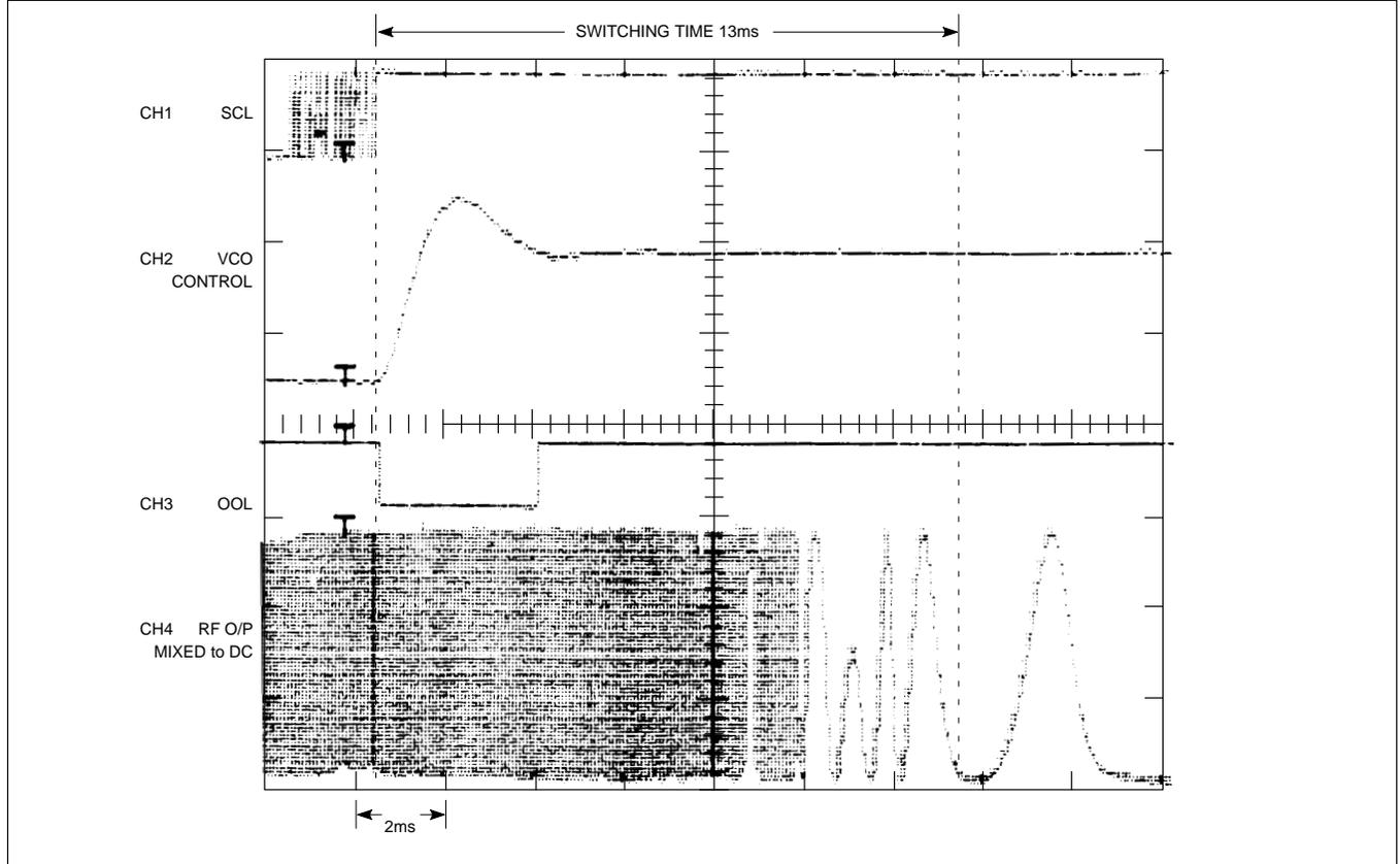
Figure 10. Typical Switching Waveforms
