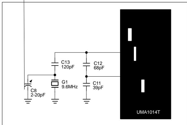
Figure 3. Crystal Oscillator Circuit Diagram
