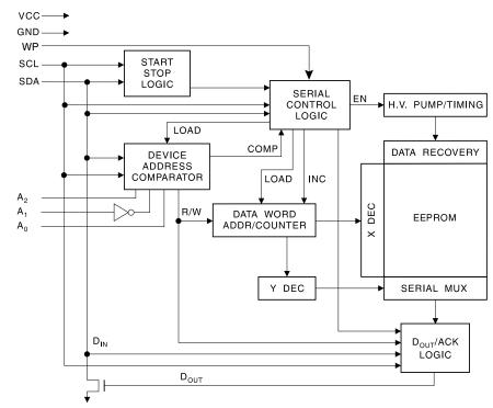
Pin DescriptionSERIAL CLOCK (SCL): The SCL input is used to positive edge clock data into each<br/>EEPROM device and negative edge clock data out of each device.
