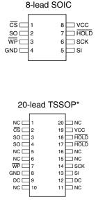
Note: \*Pins 3, 4 and 17, 18 are internally connected for 14-lead TSSOP socket compatibility.
