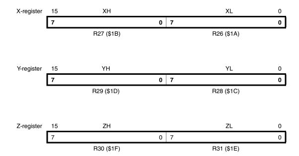
In the different addressing modes these address registers have functions as fixed displacement, automatic increment and decrement (see the descriptions for the different instructions).
