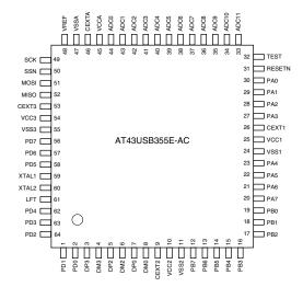
Figure 2. AT43USB355M 64-lead LQFP
