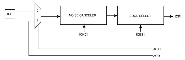
ACIC: COMPARATOR IC ENABLE ACC0: COMPARATOR OUTPUT
