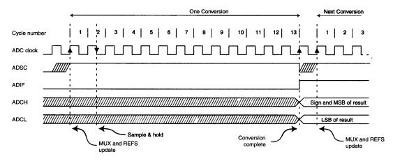
Figure 26. ADC Timing Diagram, Free Running Conversion
