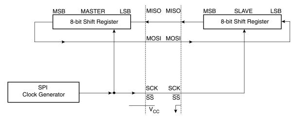
The system is single buffered in the transmit direction and double buffered in the receive direction. This means that bytes to be transmitted cannot be written to the SPI Data Register before the entire shift cycle is completed. When receiving data, however, a received byte must be read from the SPI Data Register before the next byte has been completely shifted in. Otherwise, the first byte is lost.
