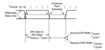
Figure 33. Receiver Jitter Tolerance
