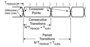
Figure 32. Differential-to-EOP Transition Skew and EOP Width
