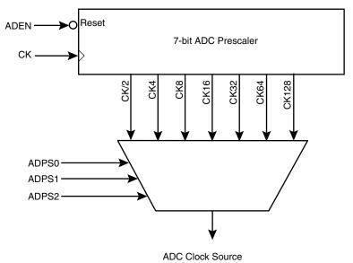
The successive approximation circuitry requires an input clock frequency between 15 kHz and 1 MHz to achieve maximum resolution. If a resolution of lower than 10 bits is required, the input clock frequency to the ADC can be higher than 200 kHz to achieve a higher sampling rate. See "ADC Characteristics" on page 66 for more details. The ADC module contains a prescaler, which divides the CK of 2 MHz clock input, to an acceptable ADC clock frequency.
