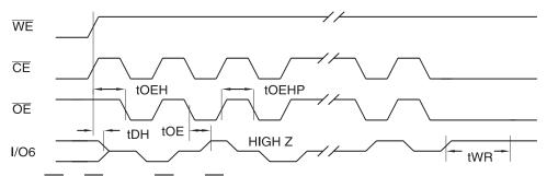
Notes: 1. Toggling either  $\overline{OE}$  or  $\overline{CE}$  or both  $\overline{OE}$  and  $\overline{CE}$  will operate toggle bit. The t<sub>OEHP</sub> specification must be met by the toggling input(s).
