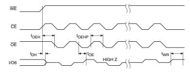
Notes: 1. Toggling either  $\overline{OE}$  or  $\overline{CE}$  or both  $\overline{OE}$  and  $\overline{CE}$  will operate toggle bit. The  $t_{OEHP}$  specification must be met by the toggling input(s).
