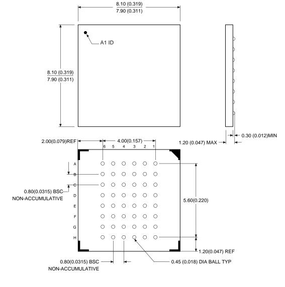
48C3, 48-ball (6 x 8 Array), 0.80 mm Pitch, 8 x 8 x 1.2 mm Chip-scale Ball Grid Array Package (CBGA) Dimensions in Millimeters and (Inches)\*
