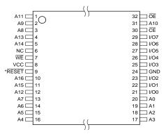
\*Note: This pin is a DC on the AT49BV001N(T) and AT49LV001N(T).
