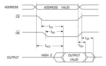
Notes: 1.  $\overline{\text{CE}}$  may be delayed up to  $t_{ACC}$  -  $t_{CE}$  after the address transition without impact on  $t_{ACC}$ .
