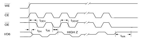
Notes: 1. Toggling either  $\overline{OE}$  or  $\overline{CE}$  or both  $\overline{OE}$  and  $\overline{CE}$  will operate toggle bit. The  $t_{OEHP}$  specification must be met by the toggling input(s).
