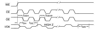
Notes: 1. Toggling either  $\overline{OE}$  or  $\overline{CE}$  or both  $\overline{OE}$  and  $\overline{CE}$  will operate toggle bit. The  $t_{OEHP}$  specification must be met by the toggling input(s).
