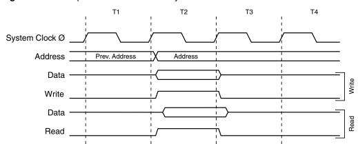
Figure 24. On-chip Data SRAM Access Cycles
