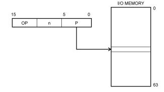
Operand address is contained in 6 bits of the instruction word. "n" is the destination or source register address.
