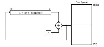
The X, Y or Z register is decremented before the operation. Operand address is the decremented contents of the X, Y or Z register.
