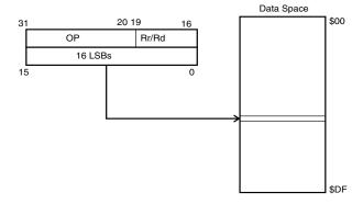
A 16-bit Data Address is contained in the 16 LSBs of a two-word instruction. Rd/Rr specify the destination or source register.
