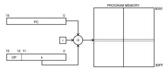
Program execution continues at address PC + k + 1. The relative address k is from – 2048 to 2047.
