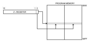
Constant byte address is specified by the Z register contents. The 10 MSBs select word address (0-1K). For LPM, the LSB selects low byte if cleared (LSB = 0) or high byte if set (LSB = 1).
