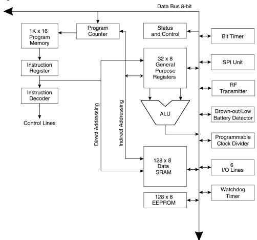
Figure 6. AVR Core Architecture
