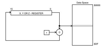
The X, Y or Z register is incremented after the operation. Operand address is the content of the X, Y or Z register prior to incrementing.
