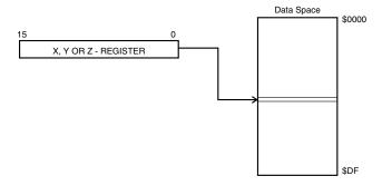
Operand address is the contents of the X, Y or Z register.
