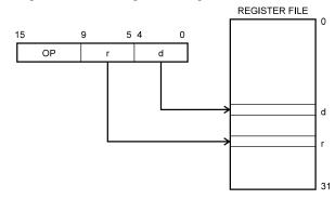
Operands are contained in register r (Rr) and d (Rd). The result is stored in register d (Rd).
