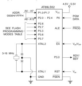
Figure 10. Verifying the Flash Memory (Parallel Mode)
