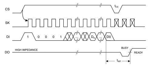
Notes: 1. Valid only at  $V_{CC} = 4.5 V$  to 5.5V. 2. Requires a minimum of nine clock cycles.
