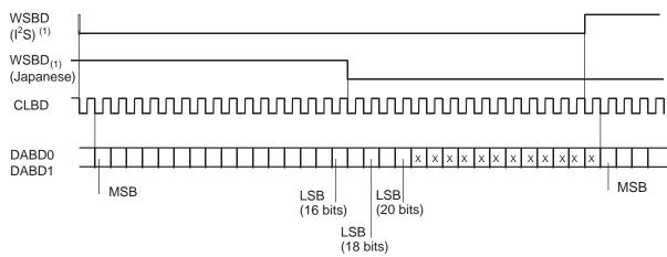
Note: 1. Selection between  $I^2S$  and Japanese format is made through DACSEL pin .
