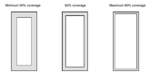
Figure 9. Solder Paste Application on Pins
