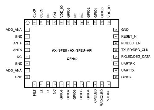
NOTE: Pins 24–26 have different functionalities in AT command and API versions, so for these pins AX-SFEU/AX-SFEU-API explanations are shown respectively.
