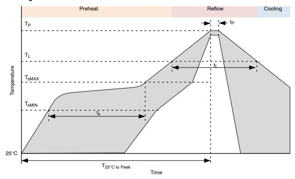
Figure 6. QFN40 Soldering Profile
