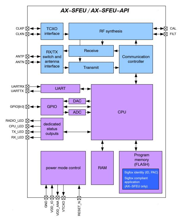
Figure 1. Functional Block Diagram of the AX-SFEU / AX-SFEU-API
