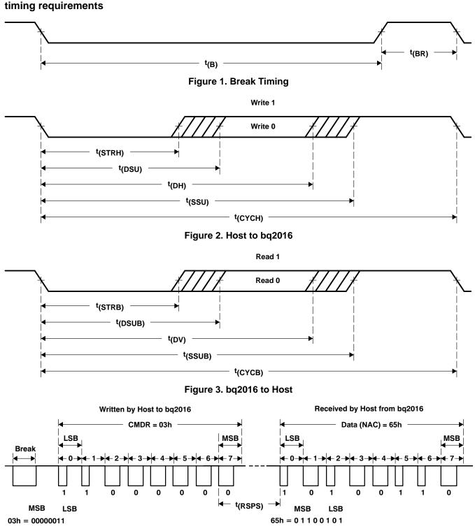
Figure 4. Typical Communication With the bq2016
