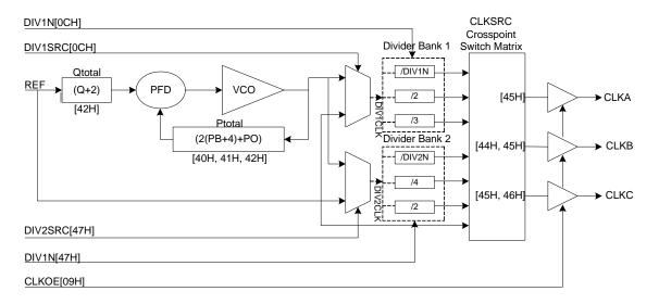
Figure 4. Basic Block Diagram of CY22801 PLL
