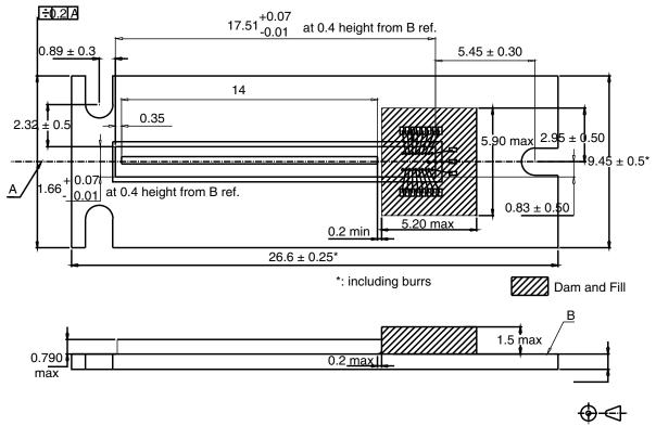
Figure 14. COB: Bottom View (all dimensions in mm)
