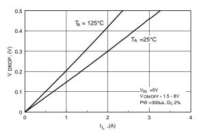
Figure 2. Conduction Voltage Drop Variation with Load Current.
