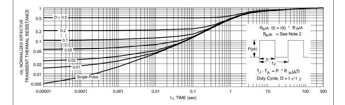
Figure 4. Transient Thermal Response Curve.
