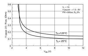
Figure 3. On-Resistance Variation with Input Voltage.
