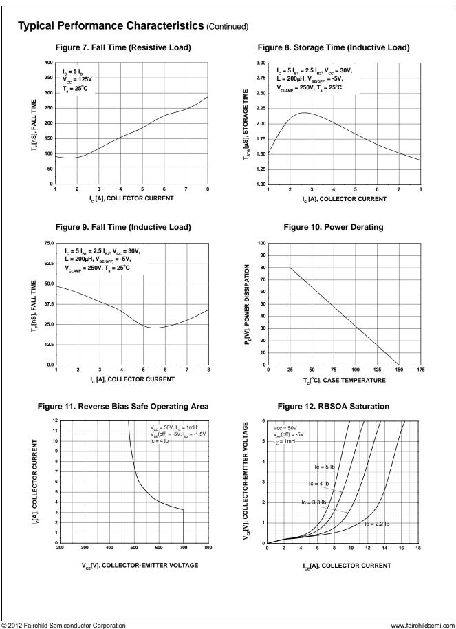
FJB3307D — High Voltage Fast Switching NPN Power Transistor
