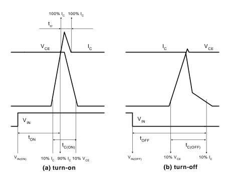
Figure 4. Switching Time Definition
