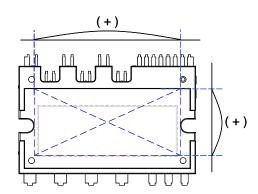
Figure 5. Flatness Measurement Position
