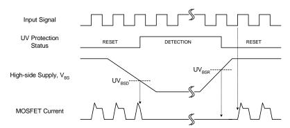
Figure 7. Undervoltage Protection (High-side)
