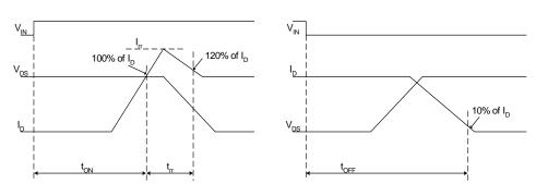
(a) Turn-on (b) Turn-off Figure 4. Switching Time Definition
