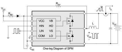
Figure 5. Switching and RBSOA(Single-pulse) Test Circuit (Low-side)
