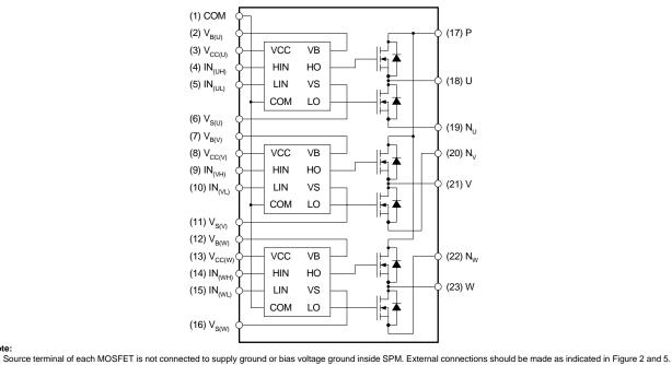
Figure 1. Pin Configuration and Internal Block Diagram (Bottom View)
