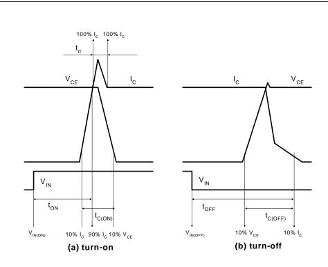
Figure 4. Switching Time Definition
