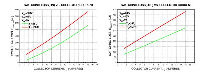
Figure 5. Switching Loss Characteristics
