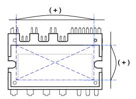
Figure 6. Flatness Measurement Position
