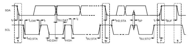
Figure 4. Definition of Timing for Full-Speed Mode Devices on the I<sup>2</sup>C Bus
