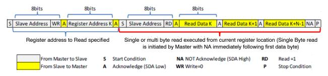
NOTE: If Register is not specified Master will begin read from current register. In this case only sequence showing in Red bracket is needed.
