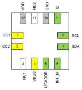
Figure 3. Pin Assignment (Top Through View)
