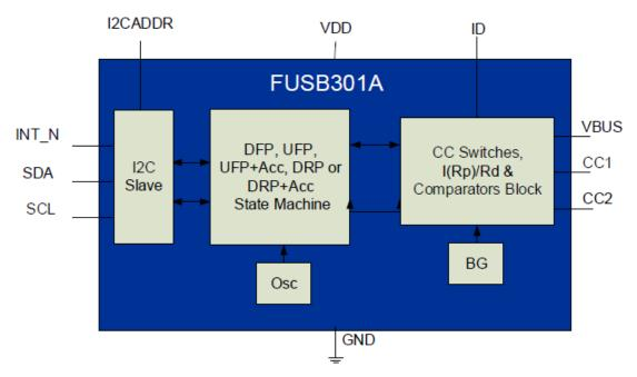
Figure 2. Block Diagram
