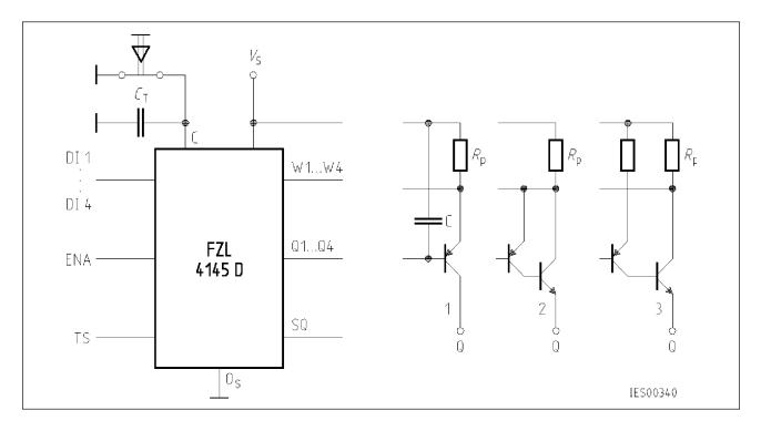
$R_{P}$  = Precision resistor (current measurement)
