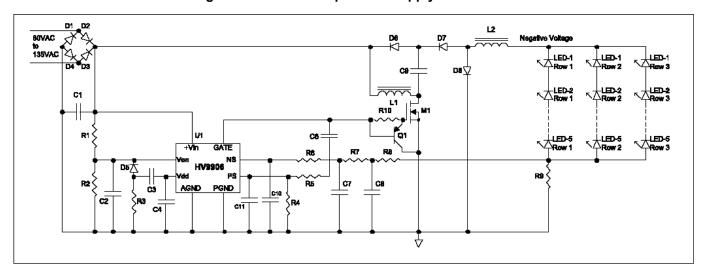
This power factor corrected circuit provides a constant average current output to power LED lamps.
