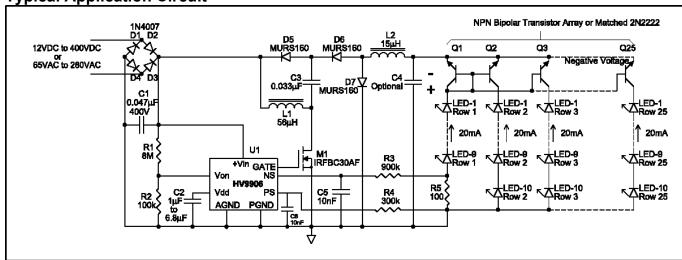
NOTE: C5 and C6 are needed for loop compensation.
