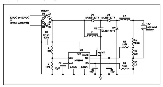
This floating battery charger circuit will charge a 6 cell 12V leadacid battery to a float voltage of 13.8V and provides a 1A charging current limit for a severely discharged or shorted battery. When the discharged battery terminal voltage is at 12V, the charging current is 130mA. The charging current decreases as the battery charges and the terminal voltage rises. When the maximum float voltage of 13.8V is reached the current into the battery will be essentially zero.
