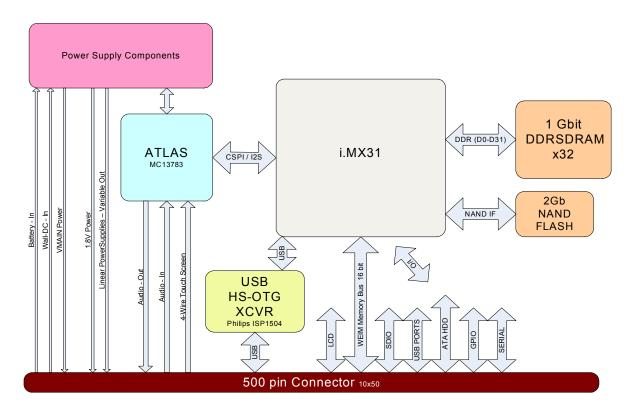
Figure 2 CPU Engine Board Block Diagram
