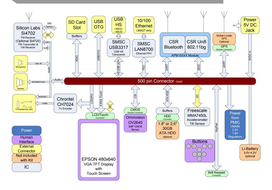
Figure 3 Personality Board Functional Block Diagram
