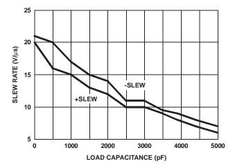
FIGURE 10. SLEW RATE vs LOAD CAPACITANCE
