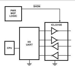
FIGURE 4. CONNECTIONS FOR MANUAL POWERDOWN
