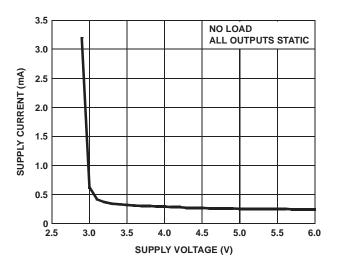
FIGURE 12. SUPPLY CURRENT vs SUPPLY VOLTAGE
