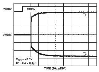
FIGURE 5. TRANSMITTER OUTPUTS WHEN EXITING POWERDOWN
