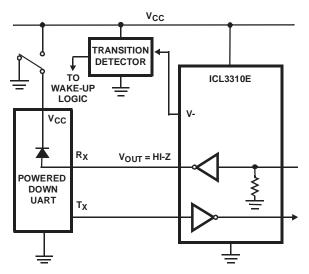
FIGURE 3. DISABLED RECEIVERS PREVENT POWER DRAIN
