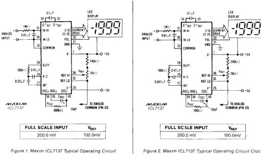
Figure 2. Maxim ICL7137 Typical Operating Circuit Clock Frequency 48kHz (3 reading/sec)
