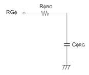
Reset gate clock equivalent circuit
