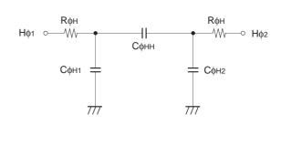
Vertical transfer clock equivalent circuit
