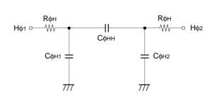
Vertical transfer clock equivalent circuit
