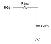
Reset gate clock equivalent circuit
