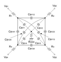
Vertical transfer clock equivalent circuit
