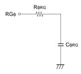
Reset gate clock equivalent circuit
