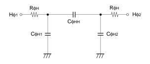
Horizontal transfer clock equivalent circuit
