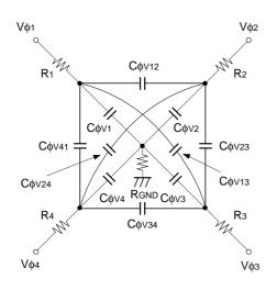
Vertical transfer clock equivalent circuit
