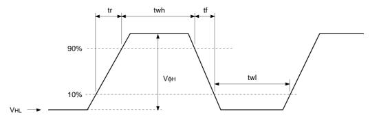
(4) Reset gate clock waveform
