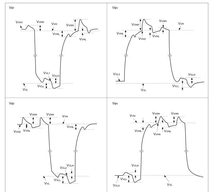
$V_{VH} = (V_{VH1} + V_{VH2})/2$  $V_{VL} = (V_{VL3} + V_{VL4})/2$  $V_{\varphi V} = V_{VHN} - V_{VLN} (n = 1 \text{ to } 4)$
