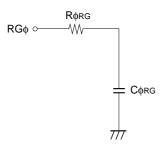
Reset gate clock equivalent circuit
