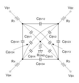
Vertical transfer clock equivalent circuit
