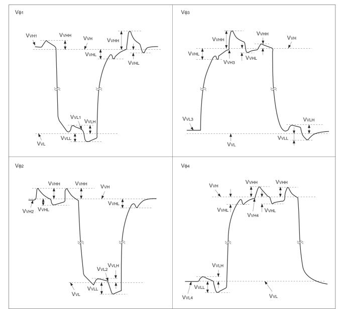
$\begin{array}{l} V_{VH} = (V_{VH1} + V_{VH2})/2 \\ V_{VL} = (V_{VL3} + V_{VL4})/2 \\ V_{\varphi V} = V_{VHN} - V_{VLN} \ (n=1 \ to \ 4) \end{array}$
