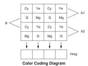
As shown in the left figure, fields are read out. The charge is mixed by pairs such as A1 and A2 in the A field. (pairs such as B in the B field)
