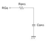
Reset gate clock equivalent circuit
