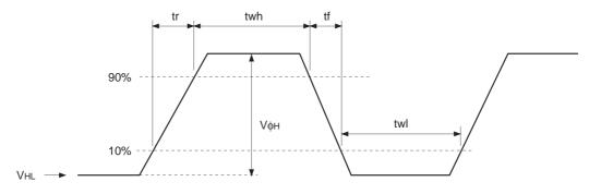
(4) Reset gate clock waveform
