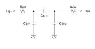
Vertical transfer clock equivalent circuit
