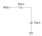
Reset gate clock equivalent circuit
