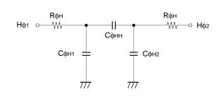
Vertical transfer clock equivalent circuit
