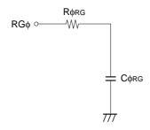
Reset gate clock equivalent circuit
