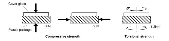
b) If a load is applied to the entire surface by a hard component, bending stress may be generated and the package may fracture, etc., depending on the flatness of the bottom of the package. Therefore, for installation, use either an elastic load, such as a spring plate, or an adhesive.
