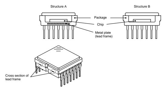
The cross section of lead frame can be seen on the side of the package for structure A.
