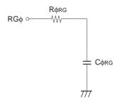
Reset gate clock equivalent circuit
