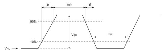
(4) Reset gate clock waveform
