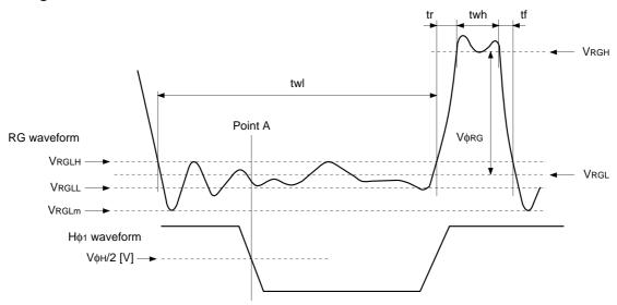
VRGLH is the maximum value and VRGLL is the minimum value of the coupling waveform during the period from Point A in the above diagram until the rising edge of RG. In addition, VRGL is the average value of VRGLH and VRGLL.
