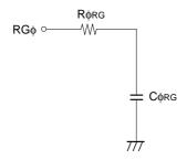
Reset gate clock equivalent circuit
