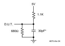
Figure 2. Output Load
