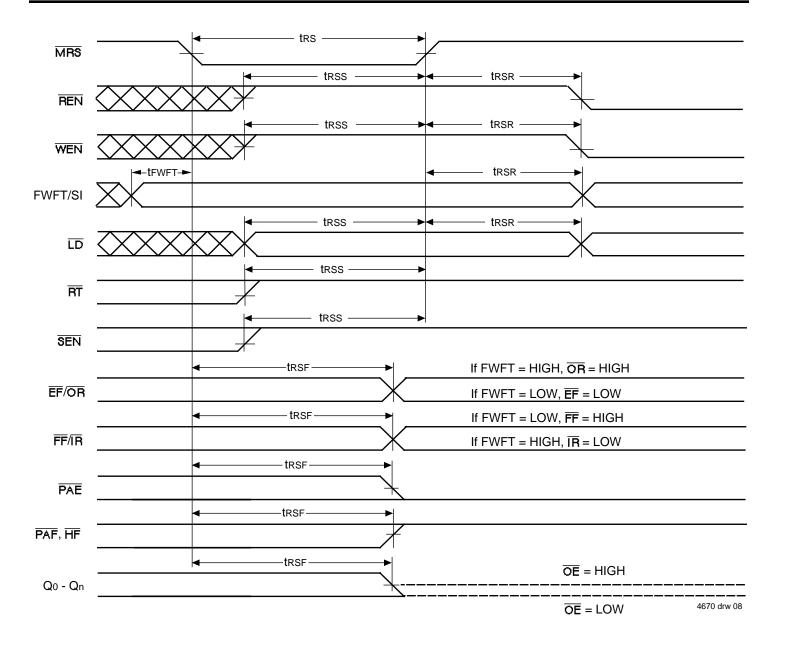
Figure 5. Master Reset Timing
