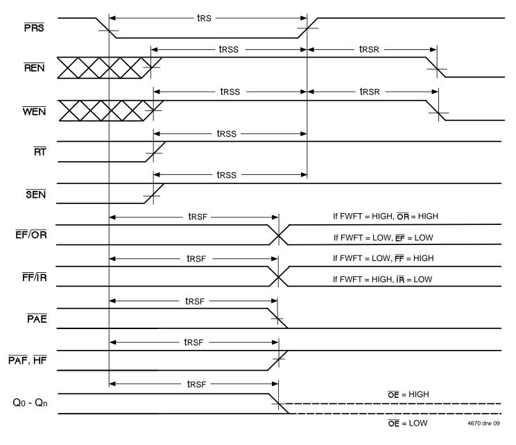
Figure 6. Partial Reset Timing
