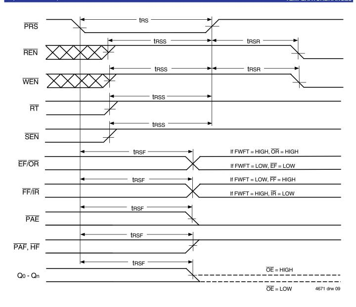
Figure 6. Partial Reset Timing
