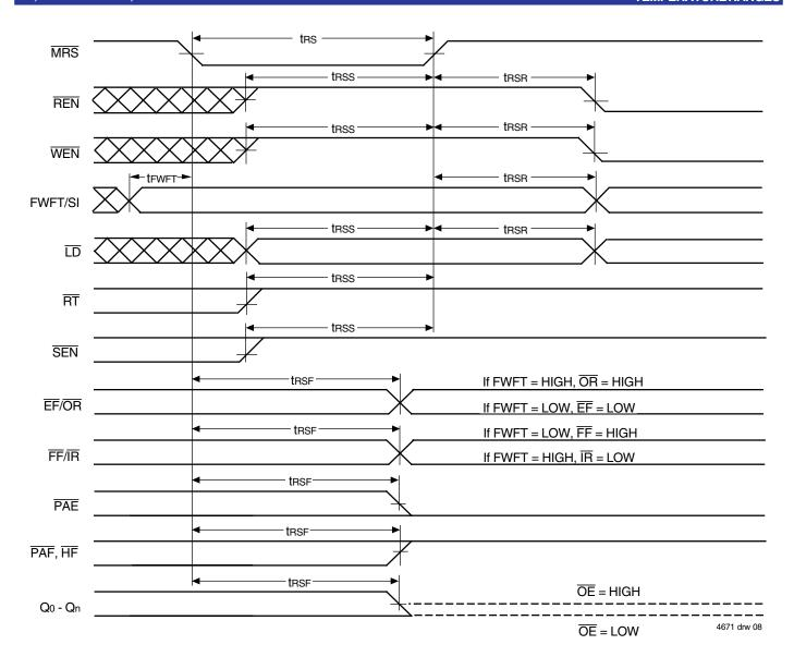
Figure 5. Master Reset Timing
