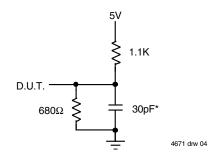
Figure 2. Output Load
