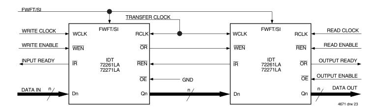
Figure 20. Block Diagram of 32,768 x 9 and 65,536 x 9 Depth Expansion
