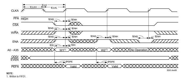
Figure 6. Port-A Write Cycle Timing for FIFO1
