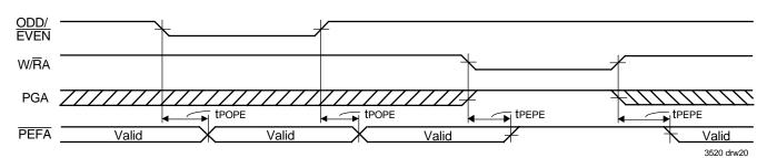
Figure 20. ODD/EVEN, W/RA and PGA to PEFA Timing
