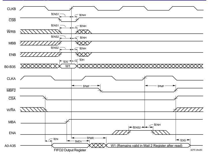
1. If Port B is configured for word size, data can be written to the Mail2 Register using B0-B17 (B18-B35 are don't care inputs). In this first case A0-A17 will have valid data (A18-A35 will be indeterminate). If Port B is configured for byte size, data can be written to the Mail2 Register using B0-B8 (B9-B35 are don't care inputs). In this second case, A0-A8 will have valid data (A9-A35 will be indeterminate).
