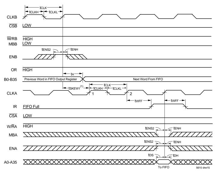
Figure 13. IR Flag Timing and First Available Write when FIFO is Full (FWFT Mode)
