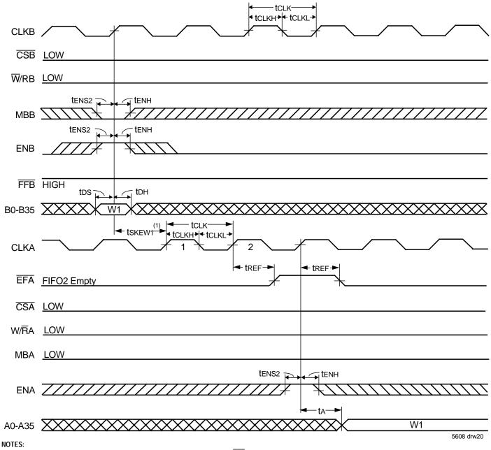
1. tskewi is the minimum time between a rising CLKB edge and a rising CLKA edge for EFA to transition HIGH in the next CLKA cycle. If the time between the rising CLKB edge and rising CLKA edge is less than tskewi, then the transition of EFA HIGH may occur one CLKA cycle later than shown.
