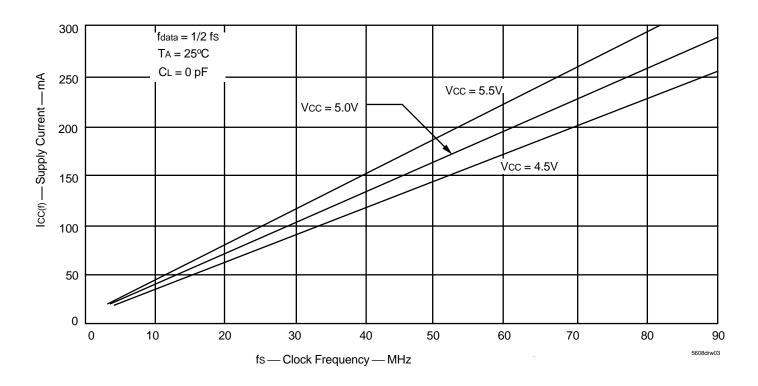
Figure 1. Typical Characteristics: Supply Current (Icc) vs. Clock Frequency (fs)
